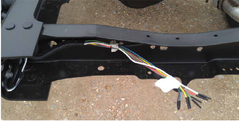
Blunt Cut Trailer Harness (can be found on trucks with OEM trailer brake controller)
