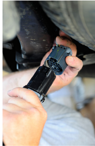
USCAR 7-way sealed plug Trailer Harness (can also be found on trucks with OEM trailer brake controller)
